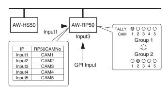
In response to inputs 1 to 5 from GPI Input, tally indicators CAM1 to CAM5 are lighted in red, and the tally ON instruction is sent to the remote cameras concerned. Only CAM1 to CAM5 serve as the GPI Input tally. This means that when a camera group other than No.1 is selected, the tally indicators will go off.
