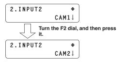
The switcher has five input lines: INPUT1 to INPUT5. Take the above steps to set the remote cameras for the input lines, and then operate the remote cameras.
